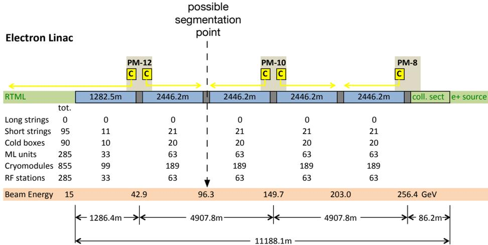
Figure 3: Possible location for the segmentation point for the Giga-Z configuration. The locations between two cryo-units avoids the need for a cryo bypass line.
