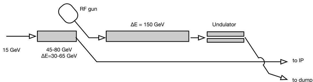
**Figure 2: "Giga Z" configuration for polarised positron production.**
