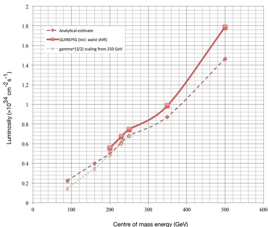
**Figure 1: ILC luminosity parameters versus centre-of-mass energy. Data points are the published numbers [1], with the exception of the 90 GeV and 160 GeV analytical points. The  $\gamma^{3/2}$  scaling (from the 250 GeV luminosity) is also shown.**
