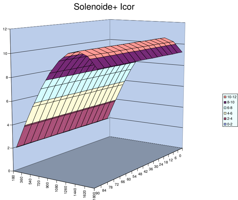
Figure 2: Configuration 2, add correction coils \int_{\ell_{\text{drift}}} \frac{B_r}{B_z} dz \simeq 10\text{mm max.}
